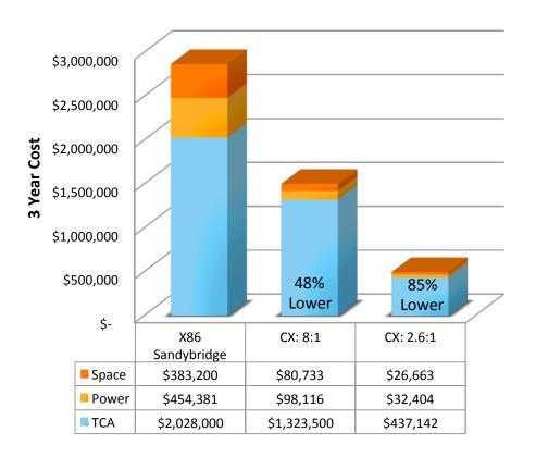
These two models reflect the 3 year cost of acquisition, power, and space of servers and networking gear for 2 different workloads, characterized by the ratio of Calxeda nodes needed to equal a dual-socket X86 server
